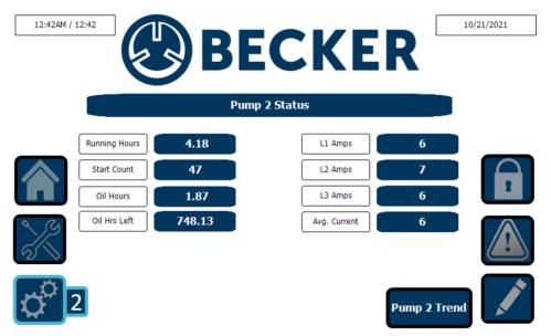
NOTE: Users must be logged in to reset maintenance hours or adjust total run hours.
