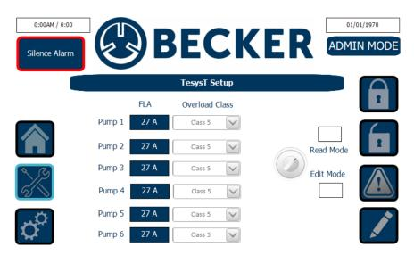
The motor settings page displays the current settings for the motor starters for each pump, such as the motor FLA and overload class. These settings are preset at the factory before shipping. If any adjustments are required, the user must first enter the correct username and password.
