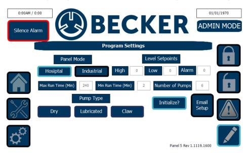
To adjust any of the vacuum setpoints or run timers, simply press the value currently displayed next to the setting you wish to adjust. Once the number pad appears, enter the new value and select "OK". If you do not wish to change the value of the selected setting, select "ESC" to return to the settings page.
