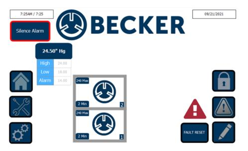
Each pump and its corresponding data are grouped into boxes. Pumps entered into the system are represented by the pump symbol and can be matched to the correct pump by the identification number shown. The status of each pump is indicated by the color of the pump symbol, as represented in the table below.
