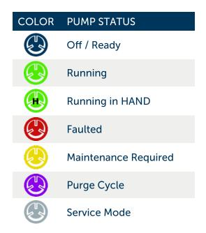
PROCEDURE: To remove a pump for maintenance/service, enter the password and locate the correct pump on the home screen. Press the pump symbol and follow the on screen prompts. While in service mode, the pump is removed from the PLC's lead/lag sequence. Additionally, an electrician or other qualified personnel may carefully switch off the pump's motor disconnect. Select the pump symbol again to remove the pump from service mode.
