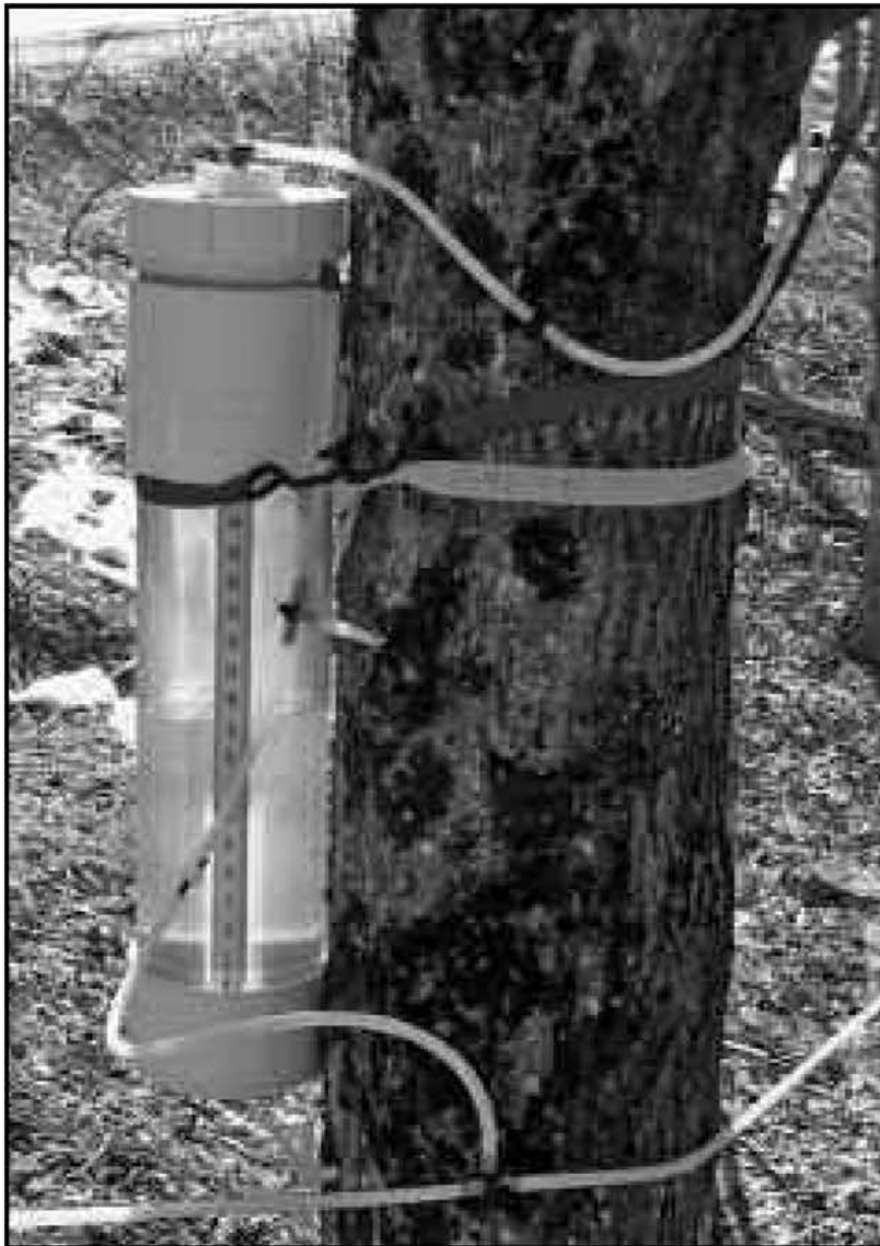
Figure 1. A chamber used to collect and measure sap volume under vacuum.
