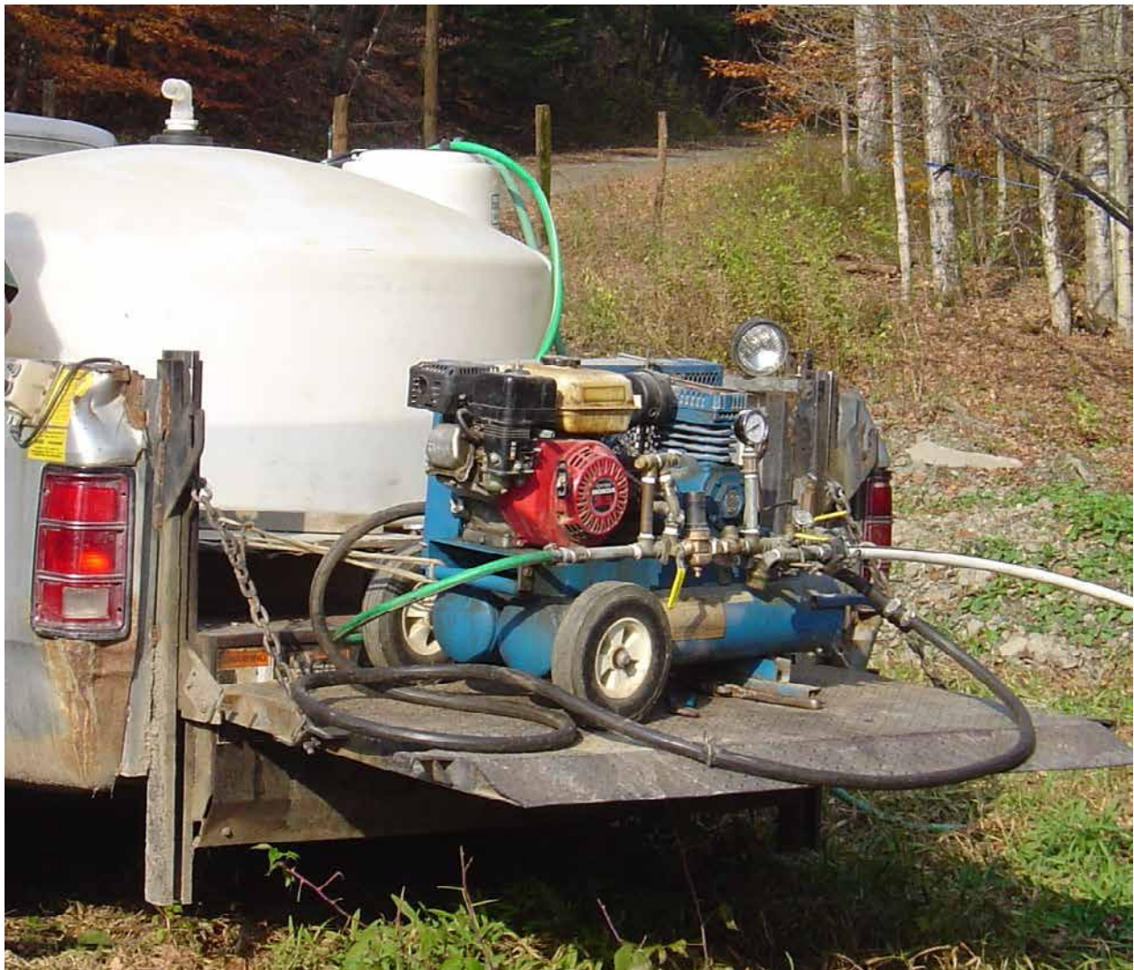
Pickup truck with water tank, air compressor and water pump set up to rinse mainlines.
