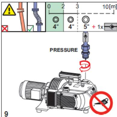
Flexible pipe should be used for pipe connections at an angle. This will prevent pipe line cracks/breakage/damage.
