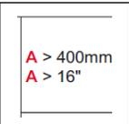
Greater than 16" (400 mm) around the pump is the distance from any object for radiant heat dissipation. Allow even more area to provide access for maintenance of the pump.
