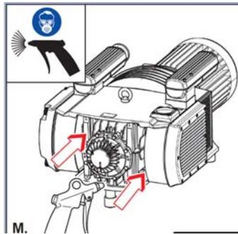
Wipe away any excess grease from the rotor shaft. (M.)
