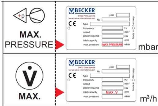
On every pump there will be the **pump nameplate**. It will state: the year the pump was manufactured, the serial number of the pump, the type of pump, frequency, rpm, kW (motor HP), volumetric flow inlet capacity, and the max pressure. The data sheet will also provide this information.
