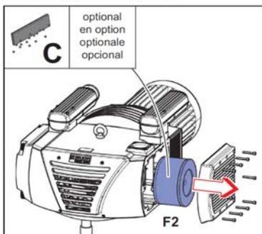
F2 is an optional dust separator, collects carbon dust for clean environment applications.
