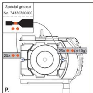
Grease bearing at 3,000 hours of run time on the pump. Locate grease gun. The push fittings are found behind the clear filter chamber cover. (O.)
