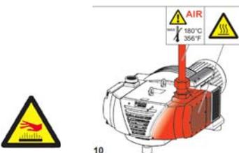
The compressor pump will become **very hot** during operation. This is normal. Care should be taken to let the unit cool down before maintenance. **(High temps: 338+ degrees F (170+ degrees C))**
