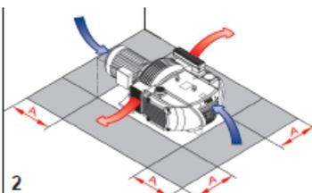
Cooling takes place by radiating heat from the surface of the pump; air flow from the fan wheel across the drive motor and from the air flow of the fan wheel on the shaft of the compressor pump.
