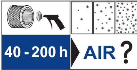
Filter/elements should be checked between 40-200 hours. The elements should be blown with compressed air from the inside out. Blast air should be felt coming through the filter/element. The element needs to be replaced if dirty or clogged. **Use only Becker Genuine filters to maintain warranty protection.**
