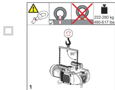
Make sure the eyebolts are fully screwed in. The position of the eyebolts fit to the center of gravity of a pump including the drive motor. If a pump without motor is to be lifted, attach another belt/rope at a suitable point.
