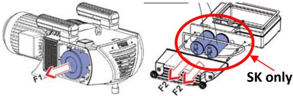
There are internal filter/elements. Every model has one behind the four knobs on the inlet side of the pump (F1). SK version only has two more filter/elements below the main inlet filter (F2).
