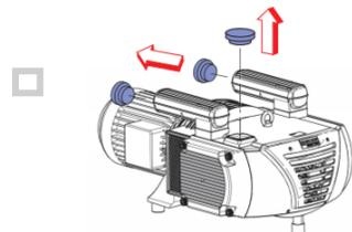
**Remove all packing materials;** cardboard/plastic covers/adhesive tape/foam from all ports and from the outside of the pump.
