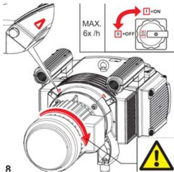
Locate the arrows that indicate correct rotation of motor/fan after electrical hook-up. Do **not reverse rotation** of the pump, this will spin the vanes backwards incorrectly and possible break or chip vanes. **Bump** the drive motor and watch the fan wheel to determine the direction.
