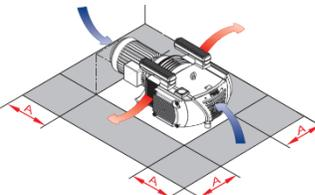
Cooling takes place by radiating heat from the surface of the pump; air flow from the fan wheel across the drive motor and from the air flow of the fan wheel on the shaft of the vacuum pump.
