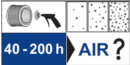
Filter/elements should be checked between 40-200 hours. The elements should be blown with compressed air from the inside out. Blast air should be felt coming through the filter/element. The element needs to be replaced if dirty or clogged. **Use only Genuine Becker filters to maintain warranty protection.**
